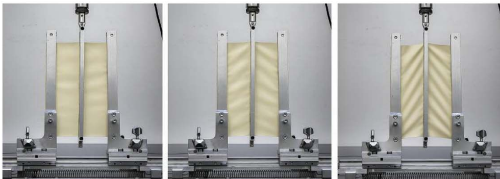
Fig. 11. The process of the shear test on the 0° direction canopy samples.
